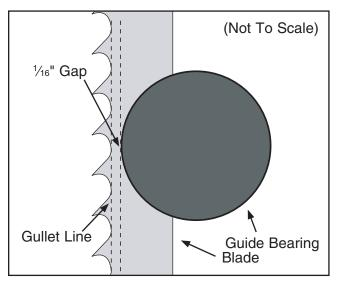
**Figure 27.** Correct guide bearing alignment against the blade.
